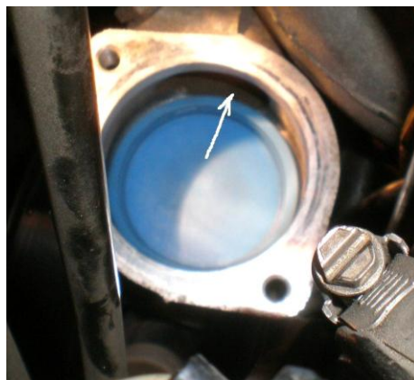
Thermostat housing with disc covering the bottom (bypass) hole Arrow points to side hole that goes to the cylinder head
