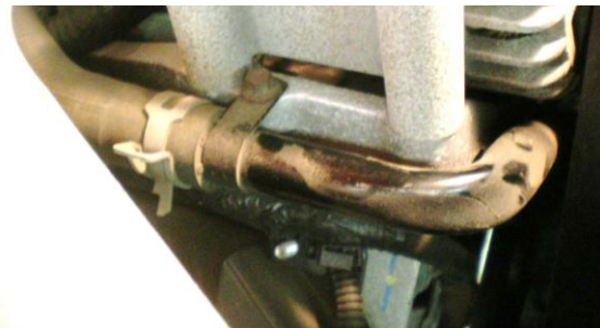
Disconnect heater hose here
